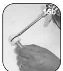
**16.** Insert bottom-out bumper and pad back onto air seal head. (fig 16a)
