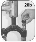
21. Spray entire spring assembly with isopropyl alcohol and wipe all grease and oil from top cap, spring and spring shaft. Apply grease to outside of entire coil spring and spring isolator.
